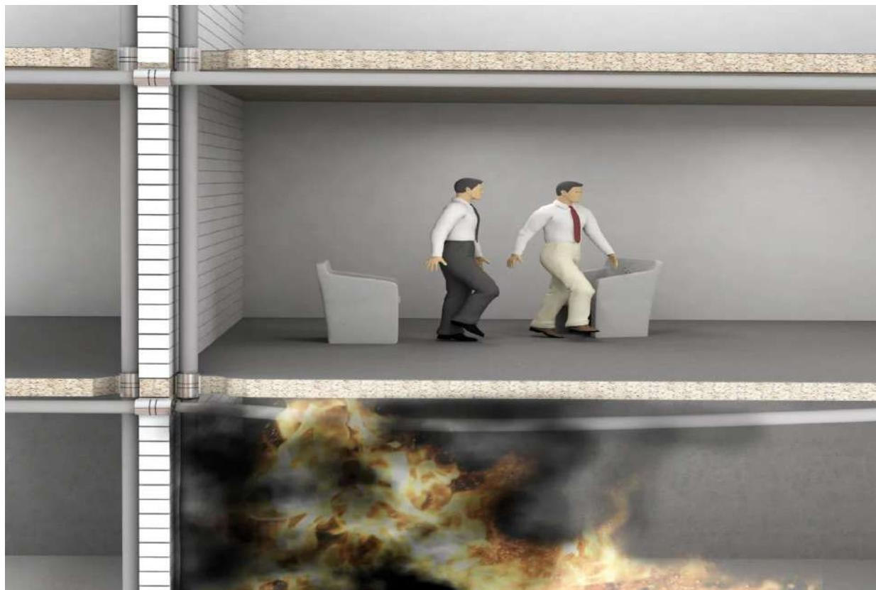
The spread of smoke and fire to adjacent areas of the building can be restricted by dividing a building into separate compartments with fire-resisting walls and floors, thereby protecting occupants and sensitive property.
